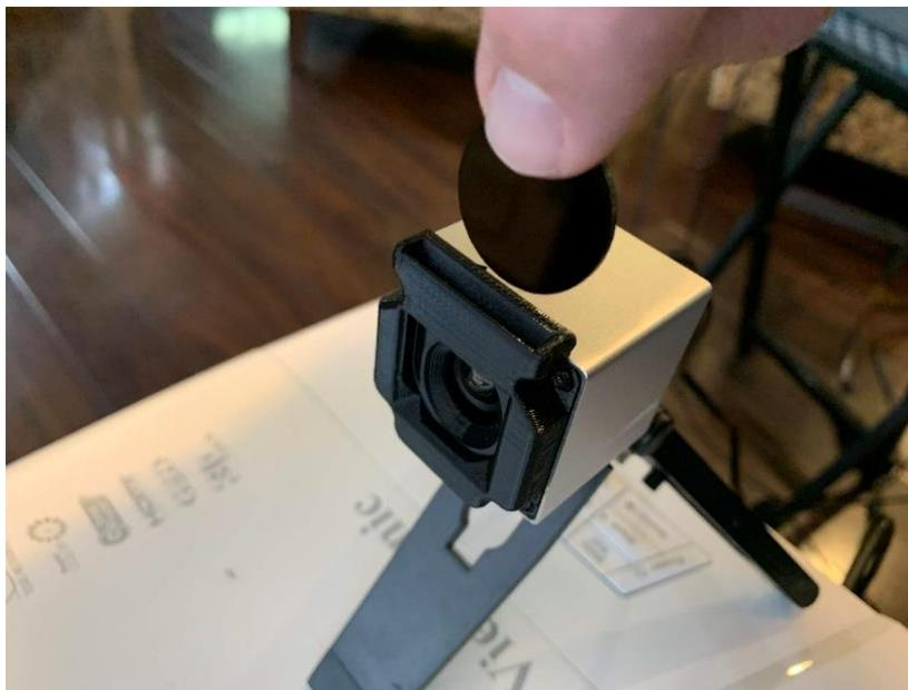
6. With the filter in place, click Continue to proceed with the rest of the calibration process. The camera will then flash some additional screens to measure the ambient light in the room and set the tracking threshold.
