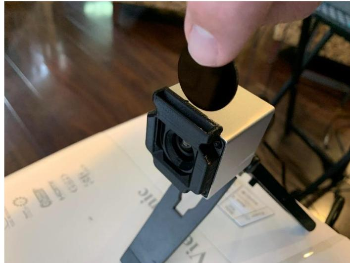
6. With the filter in place, click Continue to proceed with the rest of the calibration process. The camera will then flash some additional screens to measure the ambient light in the room and set the tracking threshold.
