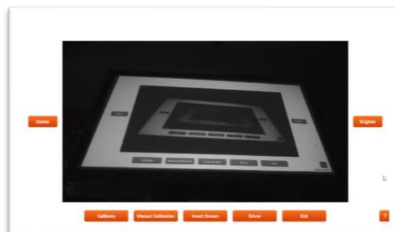
4. Now click the Calibrate button to start the calibration process. This will flash a series of dots and partial dots across the screen. It is important to not shoot a laser on the screen or walk in front of the screen during this portion.
