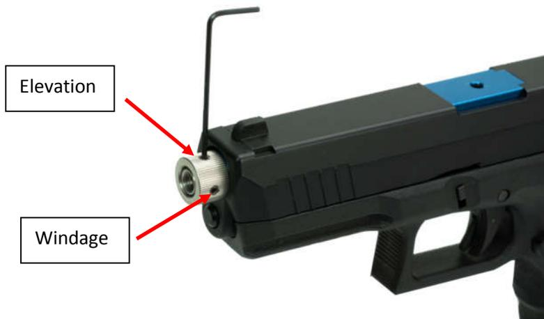
The Cartridge retainer has 4 Allen screw for adjusting your laser. By opening a screw on one side and closing the screw on the opposite side, the laser cartridge can be adjusted. The ones on the sides are for windage and the top and bottom ones are for elevation.
