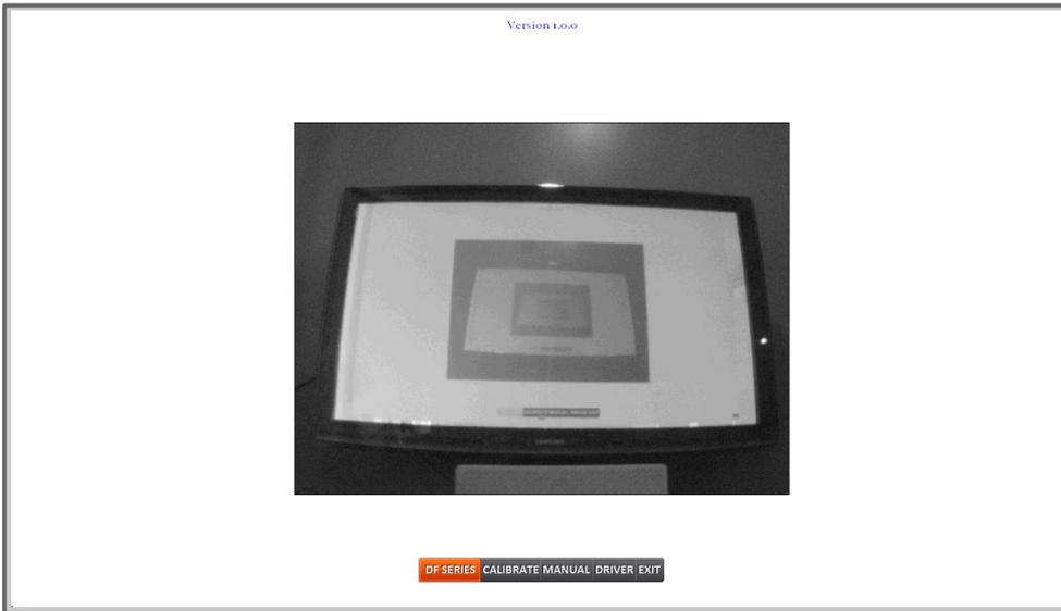
Align the camera so that the TV image fills up as much of the camera view as possible without cutting off any of the image.
