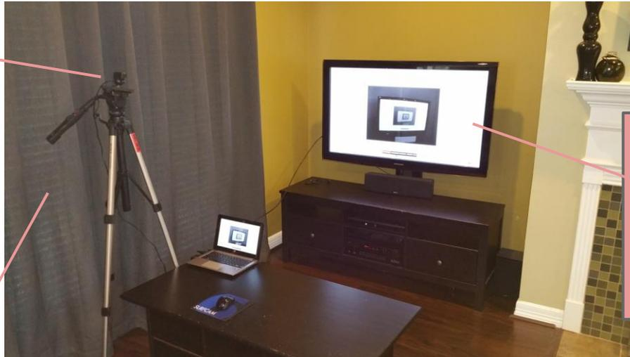
Mounting the GAMFusion filter material on the TV further eliminated the glare of reflected lighting on the TV screen and helping the laser to reflect back to the camera for accurate tracking.
